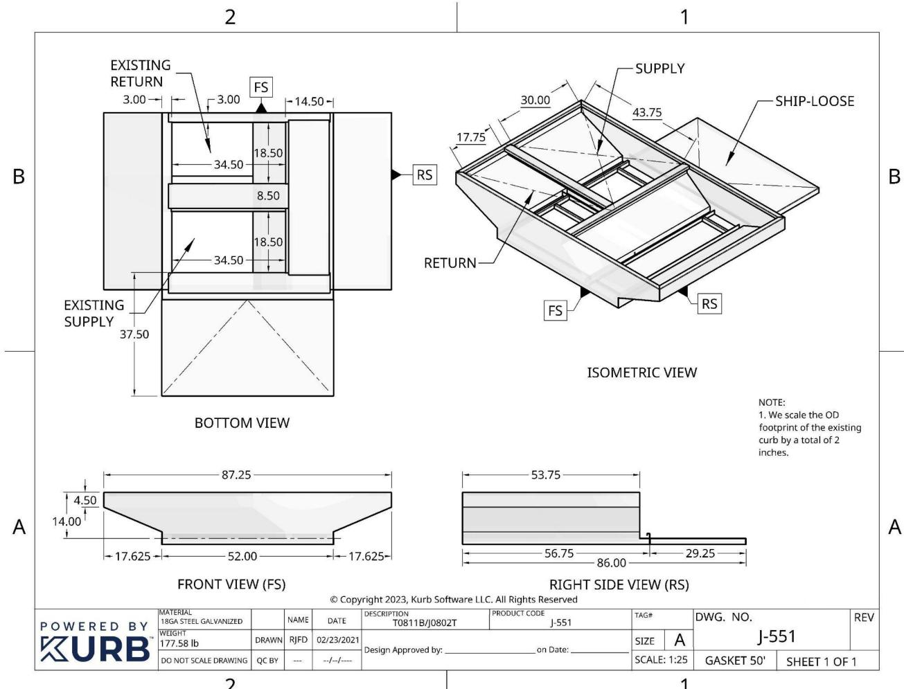
The **BOTTOM VIEW**, located on quadrant 1B, shows the dimensions for the bottom of the adapter. The **EXISTING SUPPLY** and **EXISTING RETURN** are labeled with their corresponding dimensions and positions. The location of the **Front View (FS)** and **Right Side View (RS)** are also marked as orientation guides.
